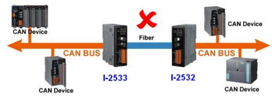
4. Use a couple of I-2533s and a couple of I-2532s. The total working distance of fiber and CAN bus will be shortened according to the baud of CAN bus.
