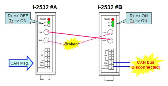
(4) One channel (Tx side) of the fiber cable is broken.
